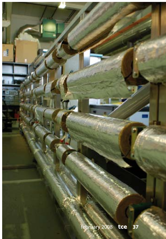
(Below left to right) Figure 3: The schematic of continuous oscillatory baffled crystalliser Figure 4: The set up of the COBC
