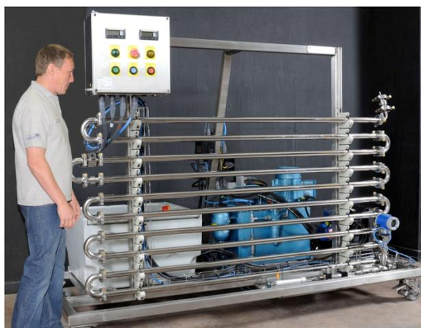
NiTech's new DN15 HP (high pressure) continuous oscillatory baffled crystalliser and reactor (COBC/COBR) offers manufacturers the opportunity to carry out a wider range of chemistries than is possible in a glass reactor.
