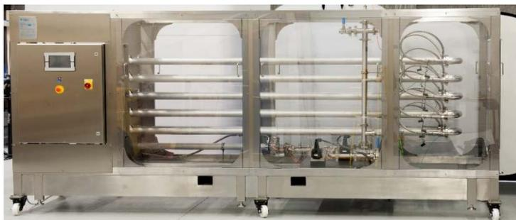
A NiTech DN43 full-scale COBR/C
