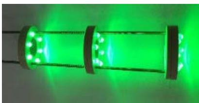
By planting LEDs on the surfaces of baffles – essential for achieving uniform mixing – this new patent enables uniform mixing and uniform light distribution (wavelength and intensity) **at all scales**. It therefore overcomes the bottlenecks of scale-up and non-uniform light distribution in full-scale photo reactors.
