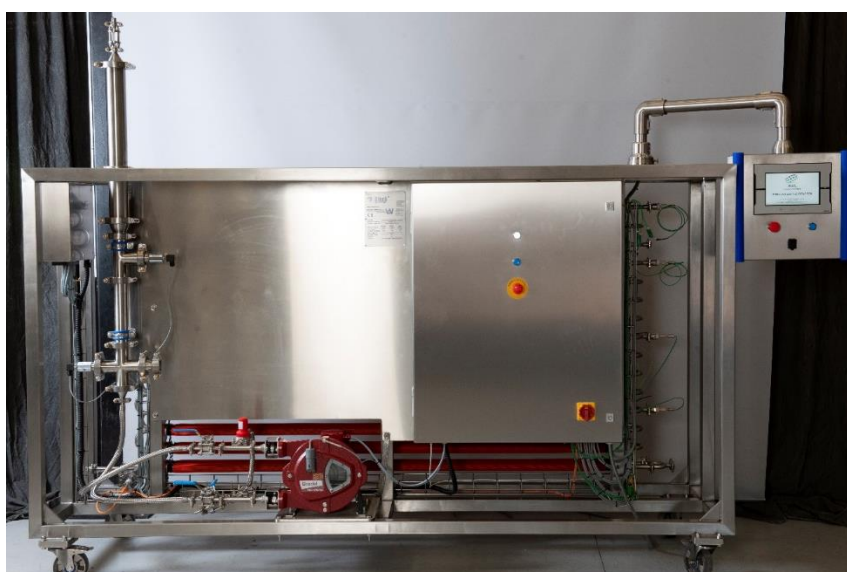
Figure 3 - The Reverse Side of a 64 m long Stainless Steel NiTech® DN15 Tubular Baffled Reactor for Enhancing Gas-Liquid Mass Transfer, showing the Liquid Pump and Gas/Liquid Separator
